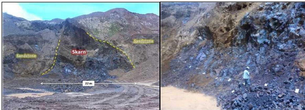
Figure 6: Massive outcropping oxidized skarn (largely hematite after magnetite) being exploited for its Fe-ore content at Kuini. Prosperity has access to the site to drill. Composite chip samples being collected across magnetite body by Prosperity staff. Analytical results from this sampling will be released when received from the laboratory.
